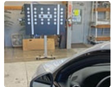
The Autel MA600 MaxiSys ADAS Calibration System's frame folds up and disassembles so that NOVUS can do calibrations in either location easily.
