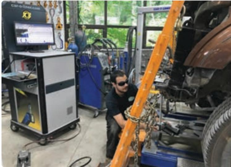
**Andrew Smith** at *Opeka Auto Repair* uses the Car-O-Tronic Vision to measure a Ford F-250 with the shop's Car-O-Liner frame machine.
